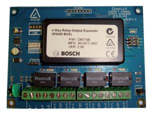
The CM710B output expansion module allows quick and easy installation of addition physical outputs to the intrusion control panel. Being LAN based the CM710B may be co-located with the intrusion control panel or remotely located.
