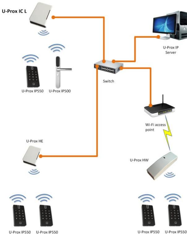
Fig. 3. An example of a local network of mixed type (Ethernet and Wi-Fi)
