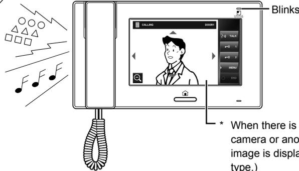
\* When there is a call from a door station without a camera or another residential station, the station type image is displayed. (The image differs from the station type.)
