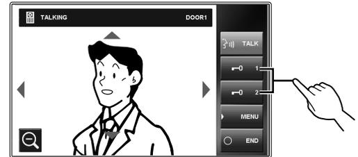
The door lock is released for the set door release time.
