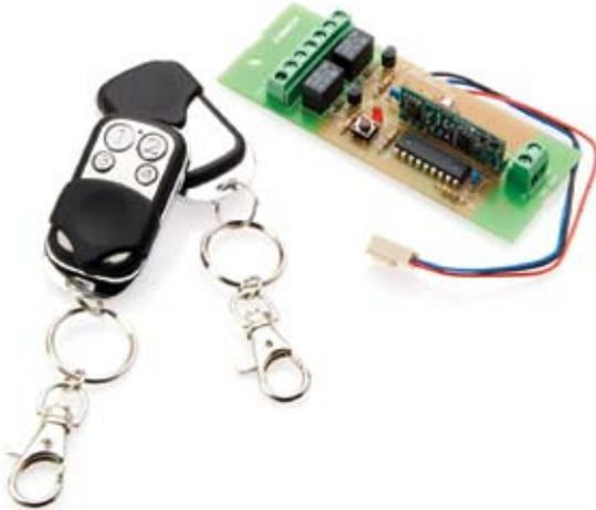
The WE800EV2 RF Arming Kit is designed to provide a convenient ON/OFF control for the Solution 800 Series alarm panels. Provision is also made for the control of up to two (2) external devices via on board relays.
